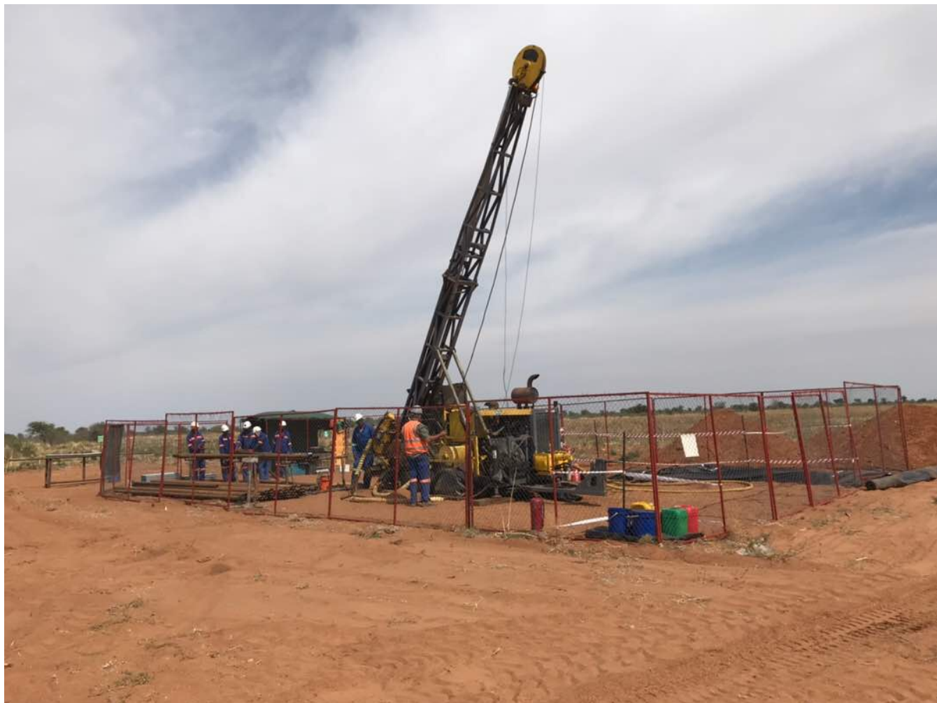
Figure 1: Photo of Diamond Core Drill Rig set up on the first hole at the KB05 exploration target.
